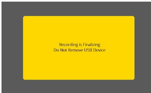
Yellow means that the recording is finalizing. **DO NOT** remove USB during this time also.
